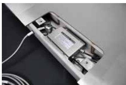
PT-S features IP66-rated protection from moisture and dust
