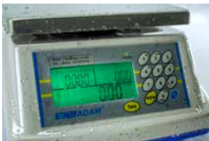
IP66-rated for protection against water and dust
