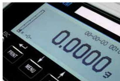
Selectable digital filtering helps minimize effects of vibration and disturbances
