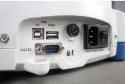
USB host for memory card, USB I/O and RS-232 interfaces
