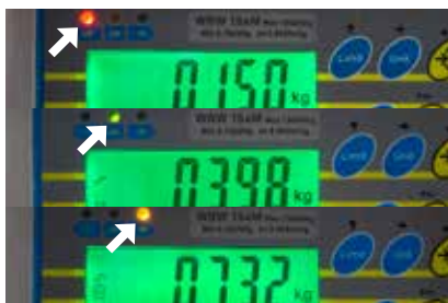
Checkweighing LEDs clearly show under, over and acceptable limits
