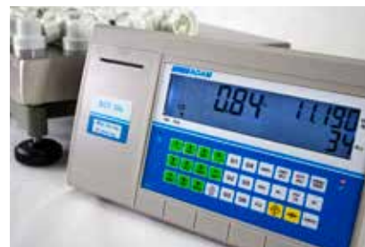
Internal counting resolution of 1:600,000 for precise results
