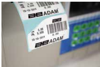
Built-in label printer allows easy output of counting data, QR codes, bar codes and more
