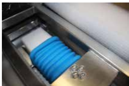
Encapsulated, silicone-coated loadcell is protected from water
