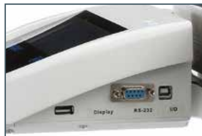
USB and RS-232 interfaces for speedy connection to printers and PCs
